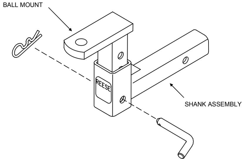
1. HITCH BALL SELECTION - Ball diameter must match trailer coupler size. The three most common sizes are 1-7/8", 2", and 2-5/16". Select ball with 1" threaded shank that is V-5 rated equal to or greater than trailer gross vehicle weight rating (GVWR).
